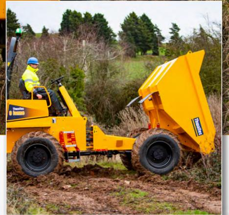
The Thwaites 9 Tonne Front Tip, Stage V dumper is manufactured with contractors and hirers in mind – ensuring operator safety, reducing risk on site, and improving performance. Front Tip dumpers allow the machine to be easily and safely unloaded, with a straightforward tipping action that places the full bucket of spoil exactly where it is required.
